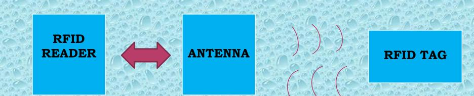
RFID technology is used for identification and to authenticate tags that are mounted in any product or individual
